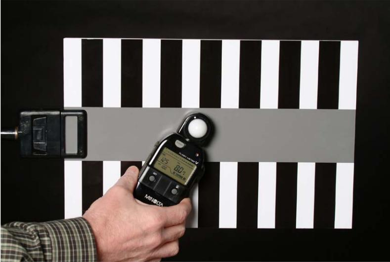
11. Adjust the sensitivity of the meter to match the fstop of the lens. (in this case f 8) Refer to the owner's manual for your meter for instructions.
